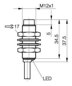
**Inductive Sensors** BES 516-3019-E4-C-PU-05 M12x1 x 37.5 normally-closed Sn=4mm unshielded
